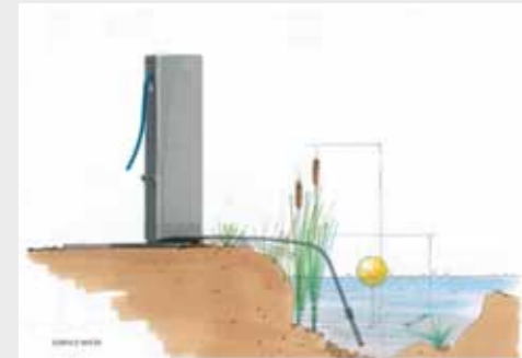
VILLAGEPUMP 500 Standard for surface water and storage tanks.
