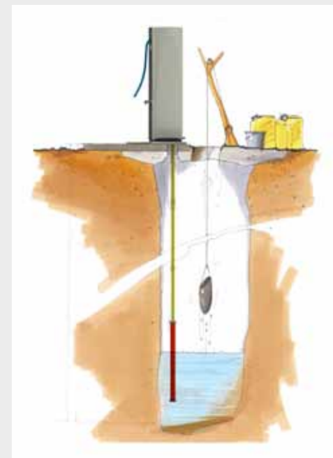
VILLAGEPUMP 500 Well for wells and boreholes up to 30 meters deep.
